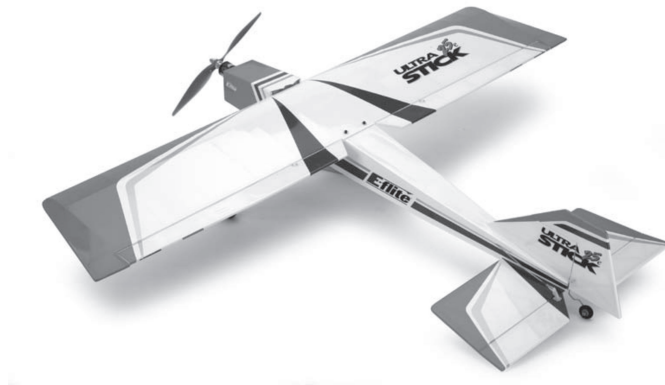
Gambar 2.1: UAV Ultrastick-25e (Sumber: horizonhobby.com, )
