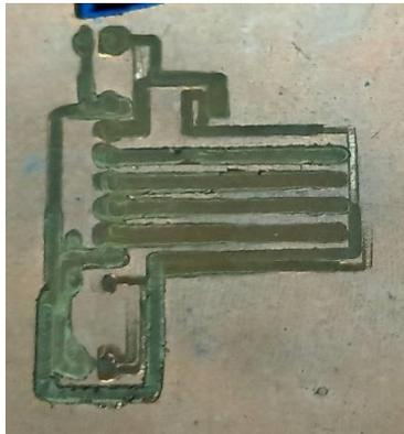
**Gambar 4.28** Hasil Gambar *Driver A4988* Dengan *Twist Bist*
