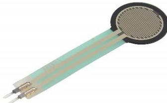
**Gambar 2.8** *FSR* Sensor
