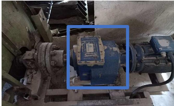
**Gambar 3.10 gear reducer**
