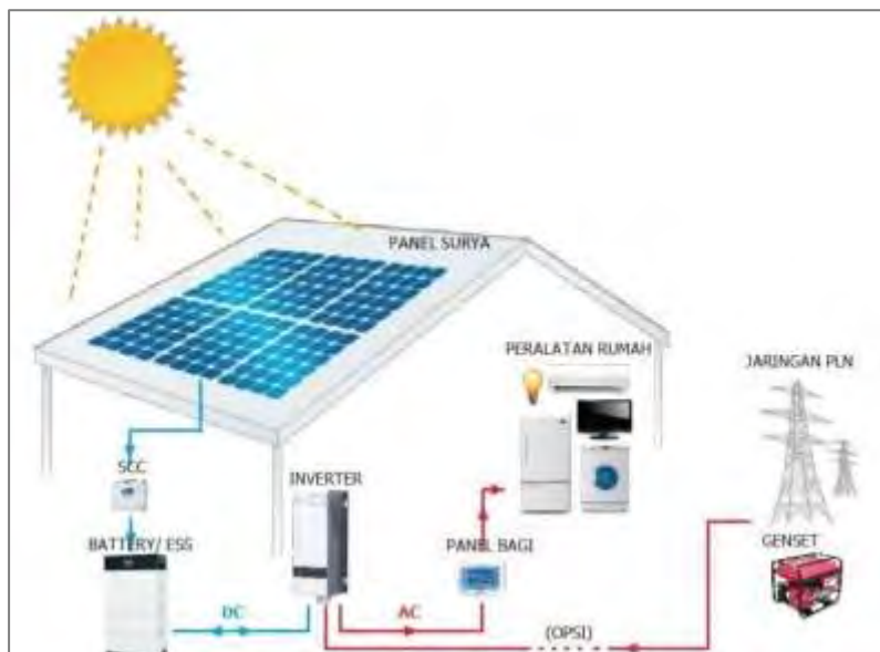
Gambar 2.14 PLTS Off-grid System
