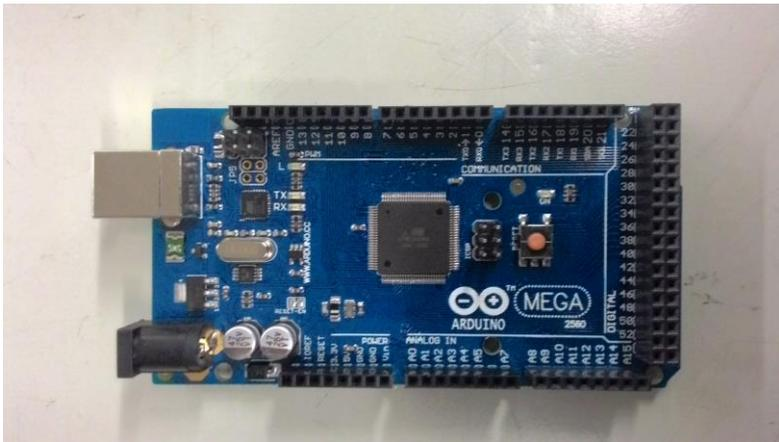
**Gambar 3.9** Arduino Mega 2560
