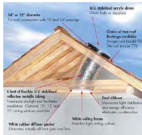
Gambar 5.15 Daylight installation
