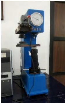
Gambar 3.5 Mesin Universal Hardness Tester HBRV - 187.5A
