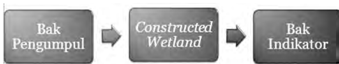
Gambar 5. 3 Diagram Alir Unit IPAL
