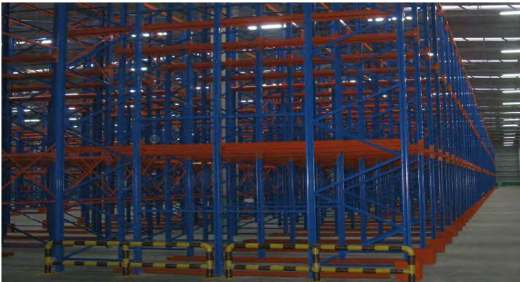
Gambar 4.1. Racking drive-in (tampak samping)
