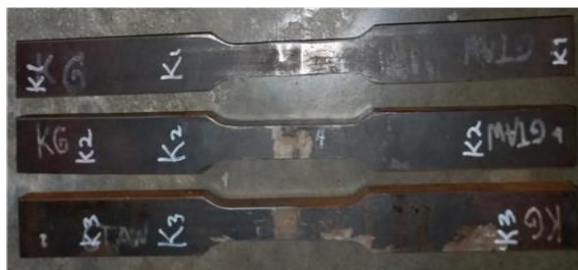
Gambar 3.14 Material Uji Tarik K Groove
