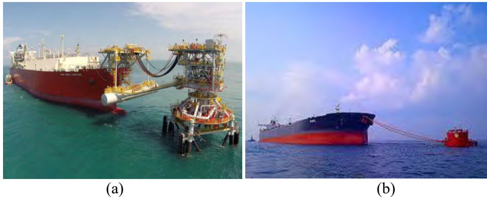
Gambar 2.1 Sistem Tambat (a) Tower Yoke Mooring System ; (b) SPM (Sumber: Helmidadang, 2012)
