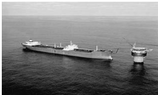
Gambar 2.6 Single Point and Reservoir (SPAR) (Sumber: Helmidadang, 2012)
