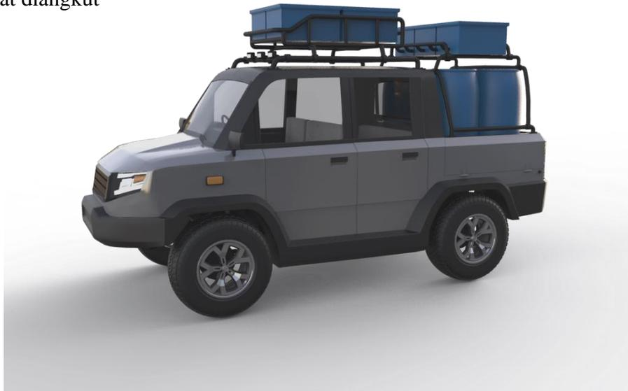
Gambar 5. 16 Skenario membawa 4 drum 120 L + 5 box 40 L
