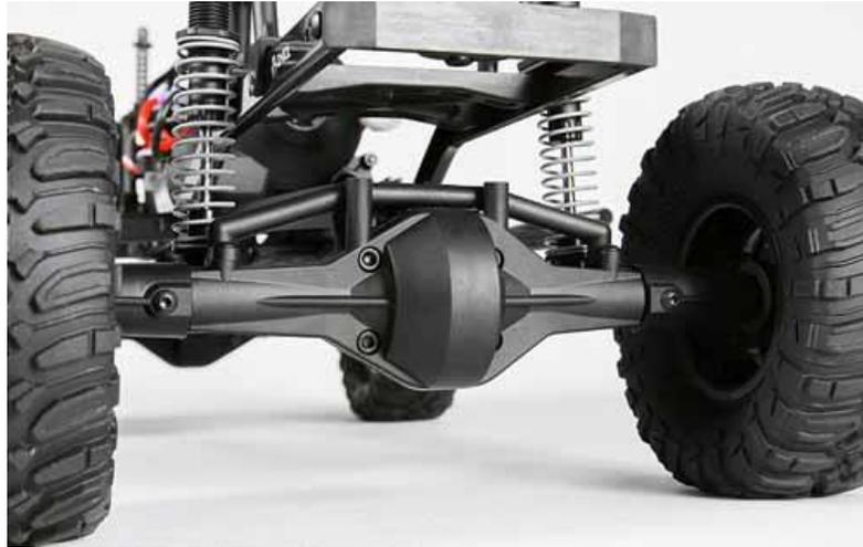
Gambar 2. 5 Rigid-Axle suspension
