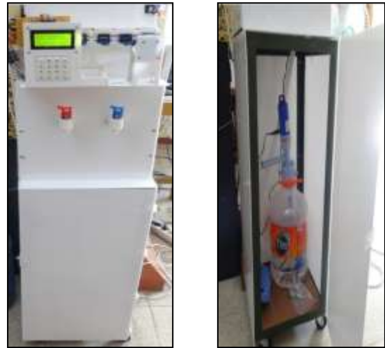
Figure 10. Smart medicine case equipped with water dispenser
