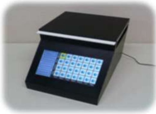
Weekly Electronic Pills Dispenser (Farcas, et.al, 2015)
