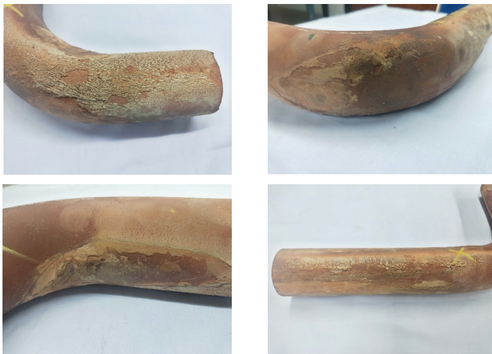
Gambar 4.6 Sampel Uji Tube Primary Superheater Elbow F10 Row 1
