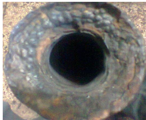
Gambar 2.12: Kerusakan tube akibat exfoliation scale oksida dan disbonding dismilliar metal weld
