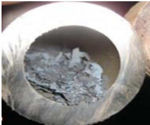
Gambar 2.12: Kerusakan tube akibat exfoliation scale oksida dan disbonding dismilliar metal weld
