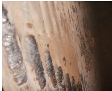
Gambar 2.12: Kerusakan tube akibat exfoliation scale oksida dan disbonding dismilliar metal weld
