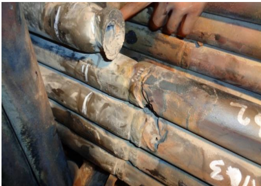
Gambar 2.13: Kerusakan tube akibat welding defects
