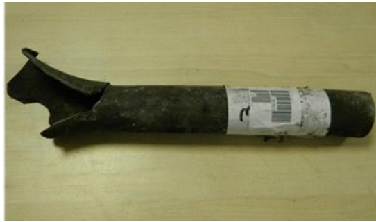
Gambar 2.12 Failure Seamless Superheater Tube (Movahedi, 2014)
