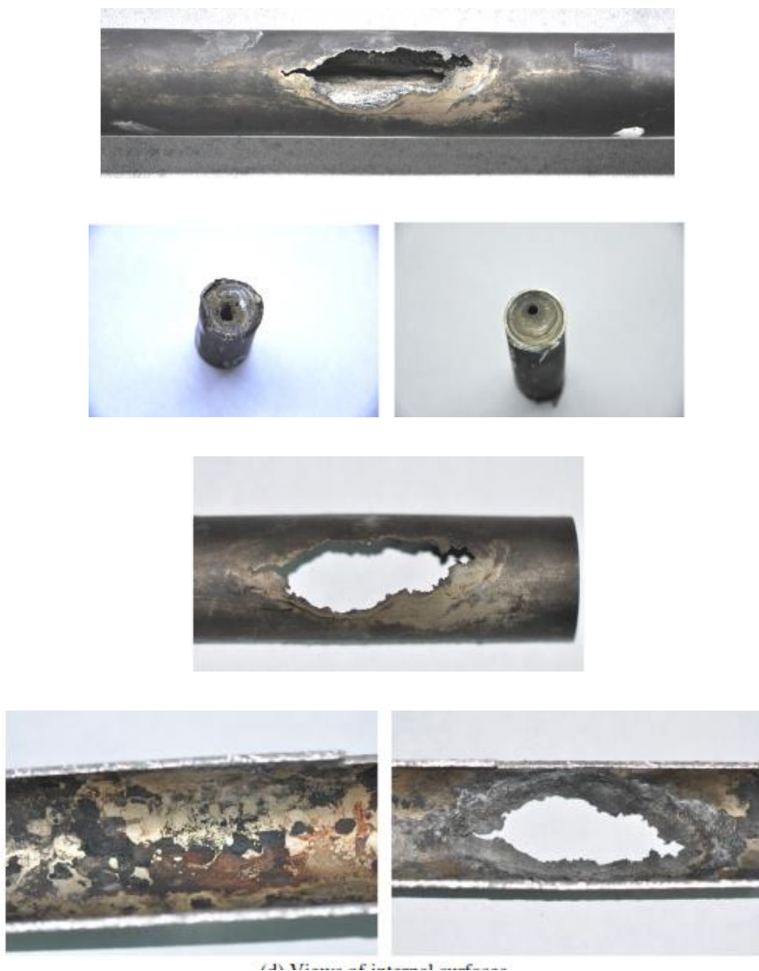
Gambar 2.11 Sampel Material Kerusakan condenser tube (H.M. Shalaby. Et al., 2011)
