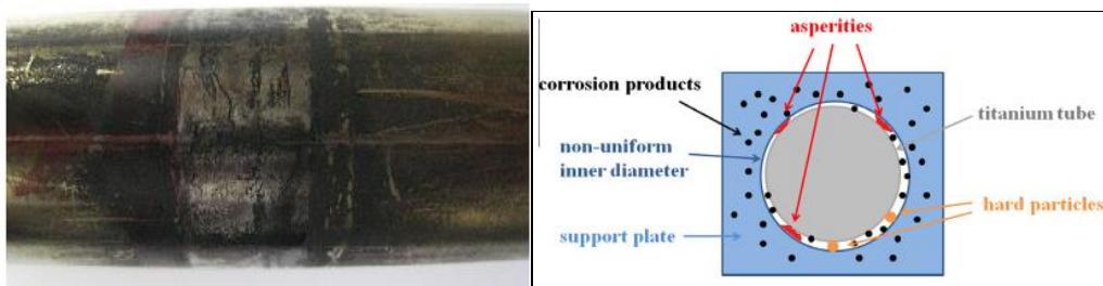
Gambar 2.15 Mekanisme wear titanium condenser tube , (Fei-Jun Chen, 2013)
