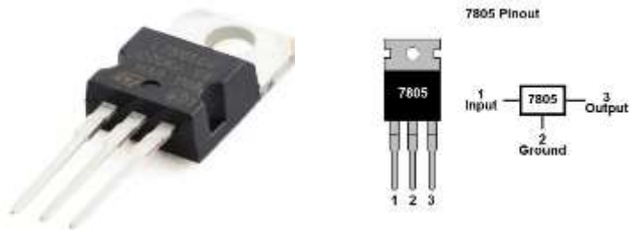
Gambar IV.11 Regulator 7805 dan pinout diagram
