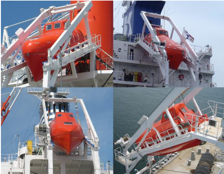
Figure 2.4 Free fall lifeboat on davit
