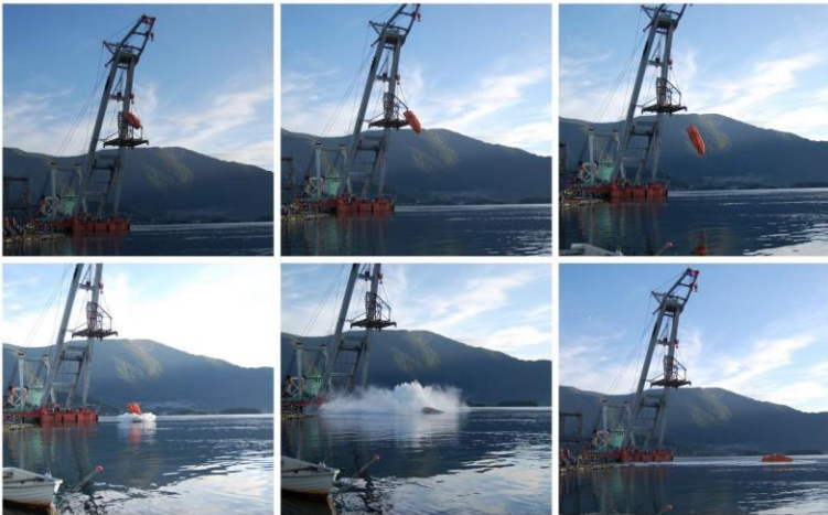
Figure 2.5 Full scale free fall lifeboat trial
