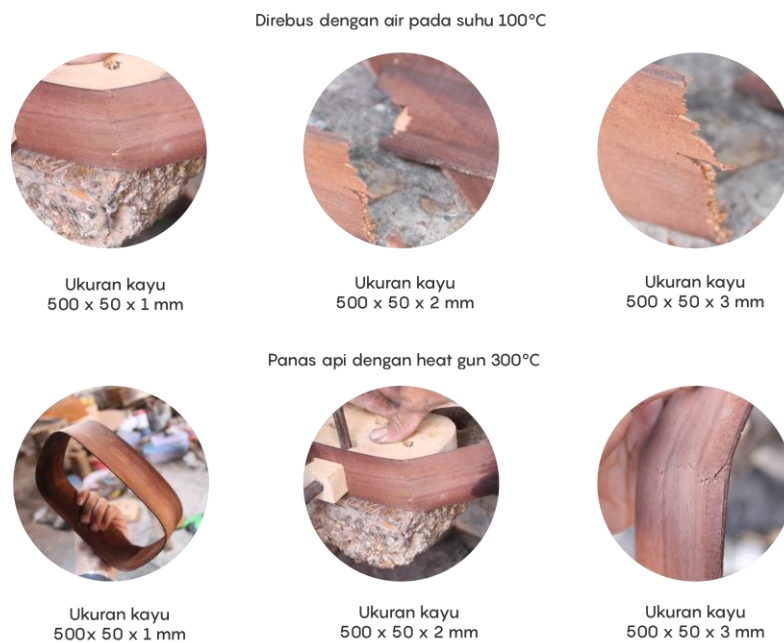
Gambar 4. 16 hasil eksperimen bending hard wood (Sesaria, 2019)
