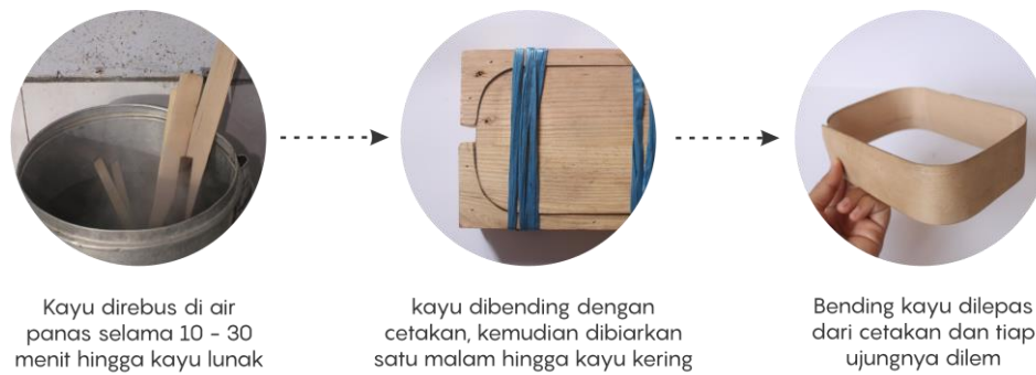
Gambar 4. 9 proses eksperimen bending soft wood (Sesaria, 2019)
