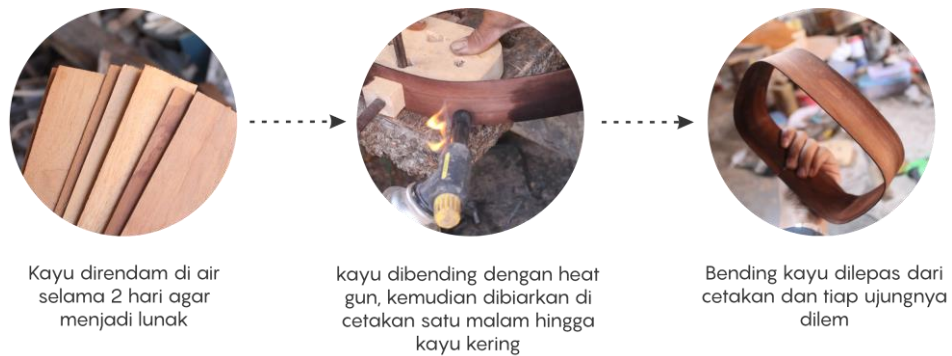
Gambar 4. 15 proses eksperimen bending hard wood (Sesaria, 2019)
