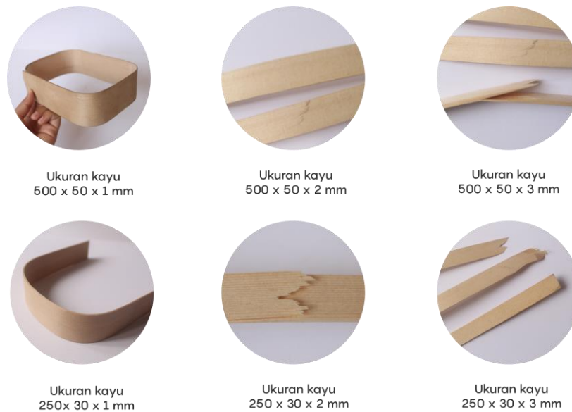
Gambar 4. 10 hasil eksperimen bending soft wood (Sesaria, 2019)
