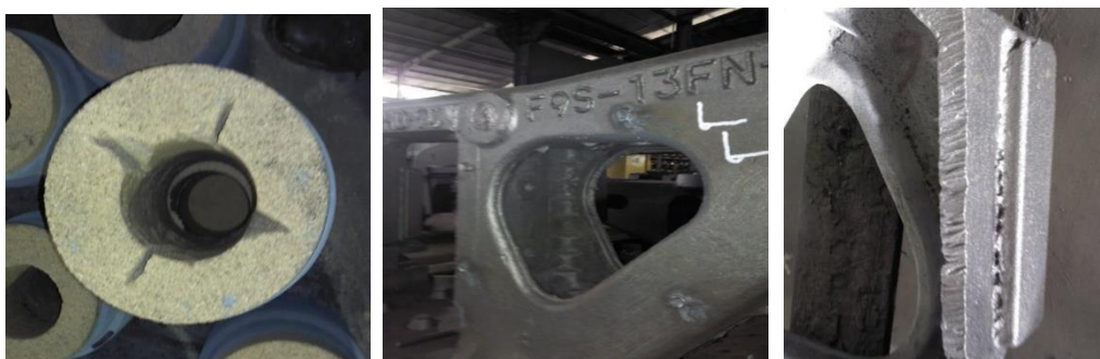
Gambar 4. 7 Contoh Defect Komponen Bogie
