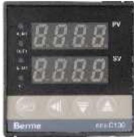
**Gambar 3.** Thermostat Berme rex-C100
