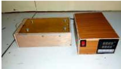
**Gambar 3.3** *Heater dan temperature control*
