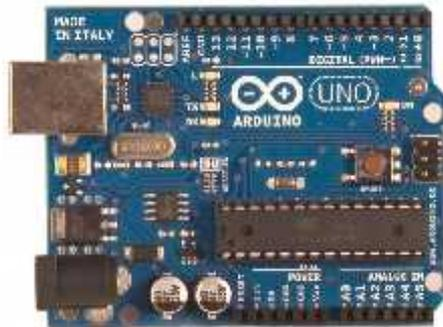
**Gambar 2.8** Board Arduino Uno
