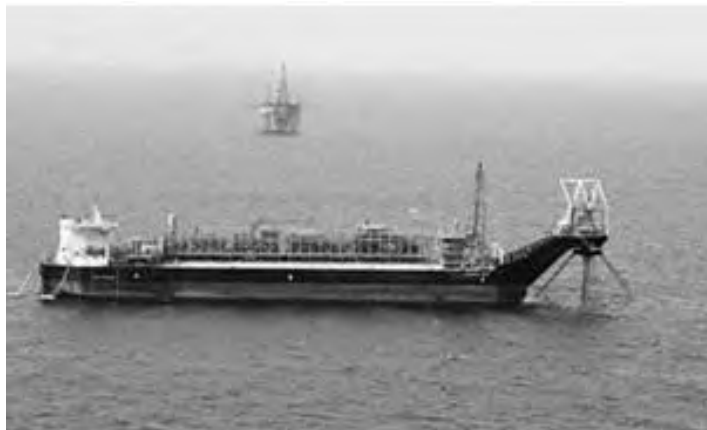
Gambar 2.14 Turret Mooring (Sumber: Helmidadang, 2012)
