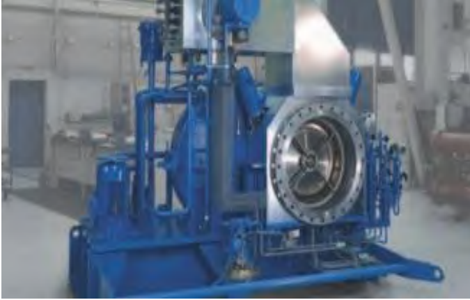
Figure 4.2 Siemens SST 060 Turbine (Source: Predesigned Steam Turbine)
