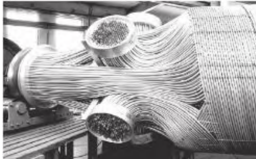
Figure 2.10 Coiled Tube Heat Exchanger II (Source Heat Exchanger Design Handbook)
