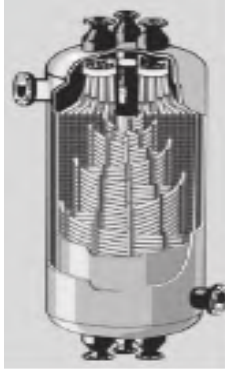
Figure 2.9 Coiled Tube Heat Exchanger I (Source Heat Exchanger Design Handbook)
