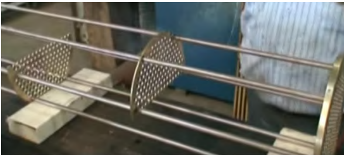
Figure 2.16 Baffle Cut (Source: Heat Exchanger Design Handbook)
