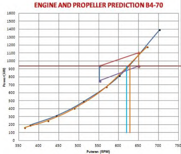
Gambar 4.7 Grafik Engine & Propeller (Rpm) Prediction B4-70
