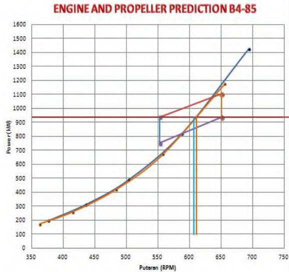
Gambar 4.14 Grafik Engine & Propeller (Rpm) Prediction B4-85
