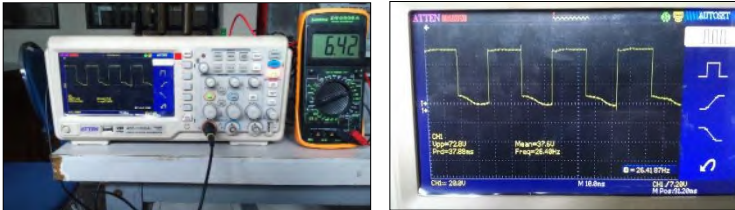
Gambar 4.2 Duty cycle PWM 55%
