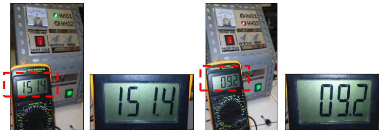
a. Arus saat relay ON
