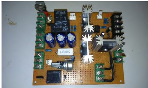
Rangkaian PWM & ON-OFF Timer
