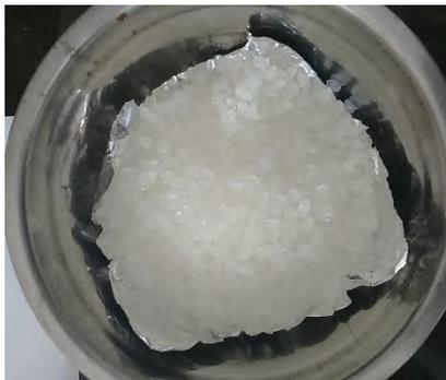
**Gambar 2.8** *Maleic Anhydride Polypropylene (MAPP)*
