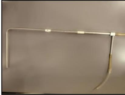
**Gambar 3.7** *Pitot Static Tube*
