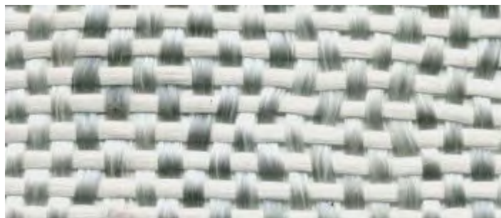
Gambar 2.1 Susunan Serat gelas Woven Roving (Carli, et al, 2012)
