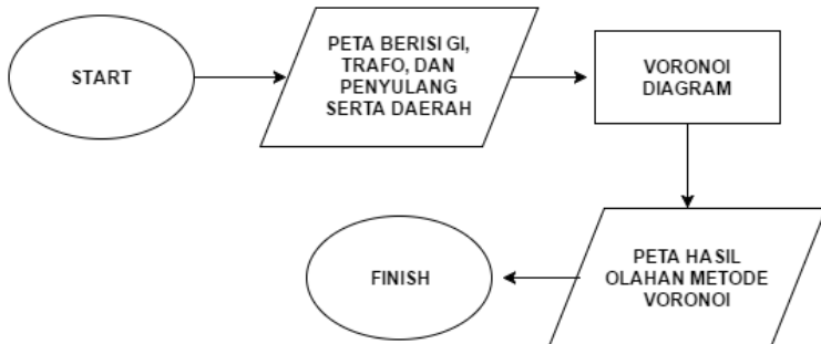
Gambar 3.1 Diagram Alur Memodelkan Voronoi Diagram
