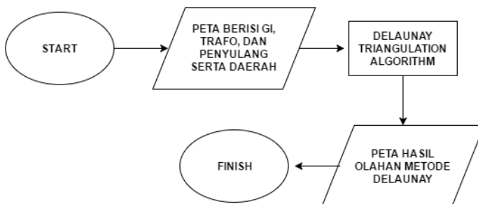
Gambar 3.2 Diagram Alur Memodelkan Delaunay Triangulation Algorithm
