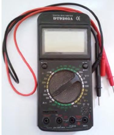
Gambar 3.3. Multimeter.
