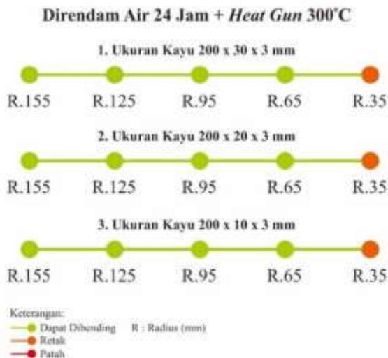
Gambar 4. 27. Perbandingan Hasil Bending Direndam Air 24 Jam + Heat Gun
