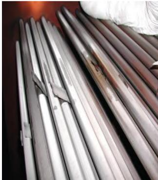
*Gambar 2.5 Steam Impingement Erosion*
