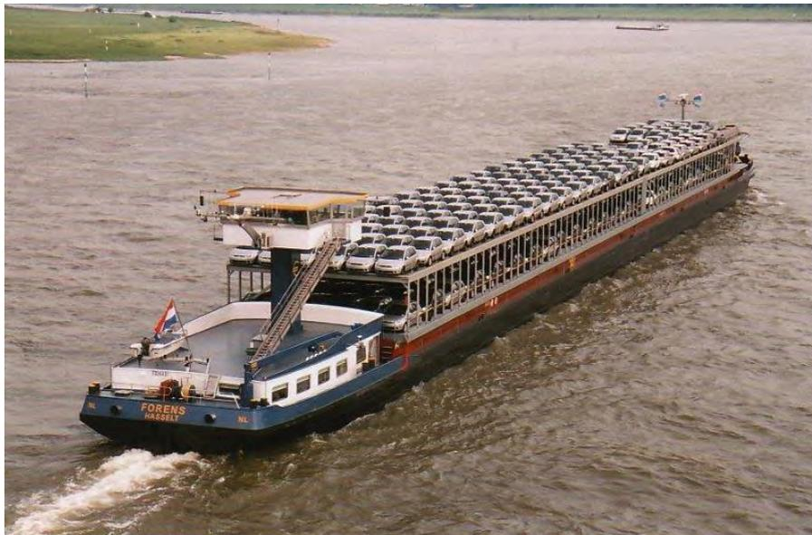
Gambar 2. 9. *Self-Propelled Car Barge* di Sungai Rhine, Jerman (Hofstra University, 2014)
