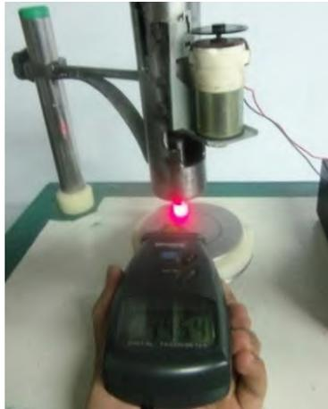
**Gambar 3.7** Kalibrasi *Speed Control*
