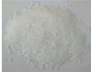
Gambar 3.4 *Maleic Anhydride Polypropylene* (MAPP)
