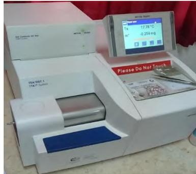
Gambar 3.8 *Differential Scanning Calorimetry (DSC)* Merk *Mettler Toledo*
