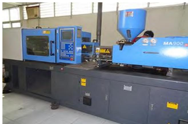
Gambar 3.9 *Mesin Injection Molding* HAITIAN-MA900/260e
