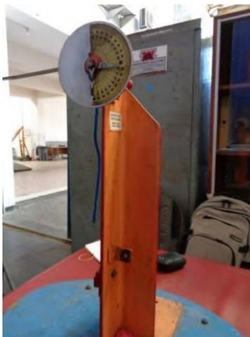
Gambar 3.12 Mesin *Mini Impact Tester* jenis *charpy*
