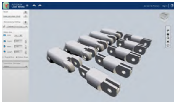
Gambar 3.15 Model 3D middle phalange dan distal phalange
