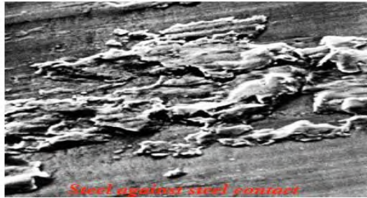
Gambar 2.20 Pengamatan Micrographs Keausan Adhesif
