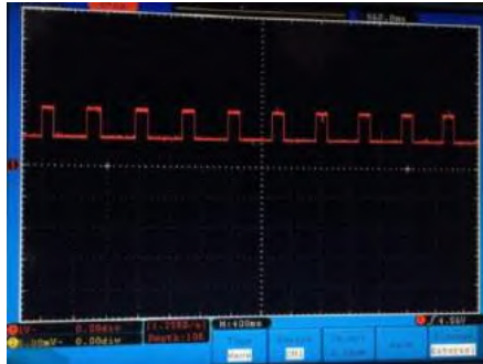
Gambar 3.20 Sinyal Tp 5 ( Output comparator ) IC LM 393
