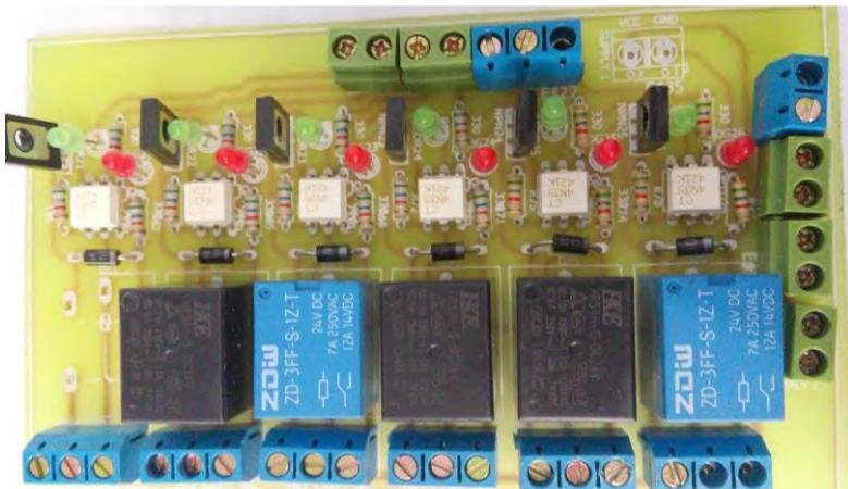
**Gambar 3.8** *Hardware Driver Relay Lampu*
