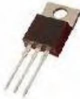
**Gambar 2.4** Transistor
