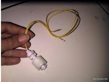
**Gambar 2.1** Sensor *Floatswitch*
