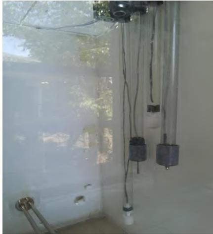
**Gambar 3.5** Sensor *Float Switch high* dan *low*
