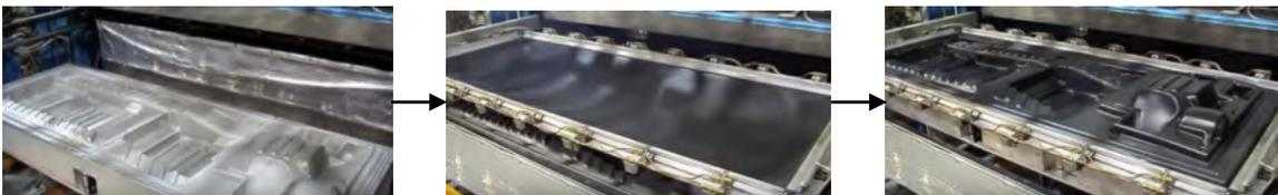
Gambar 2.9. Proses Thermoforming
