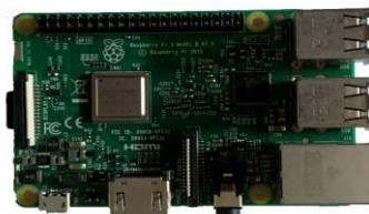
**Gambar 2.4** Raspberry Pi 3 Model B
