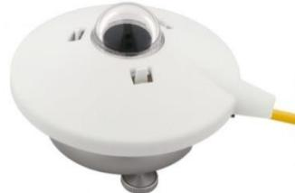
**Gambar 3. 4 Pyranometer**
