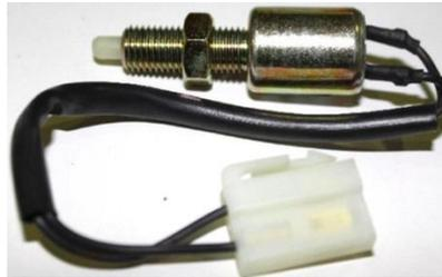
**Gambar 2.6** *Brake switch* (Automotive, 2014)
