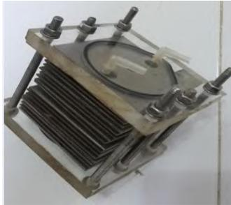
*Gambar 4.19 Generator HHO Dry Cell Sebelum Pengujian*
