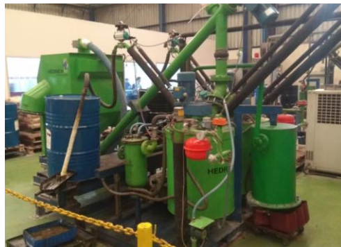
Gambar 2.16. Proses Mixing Resin
