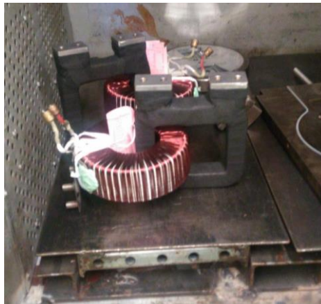
Gambar 2.14. Proses Oven Active Part
