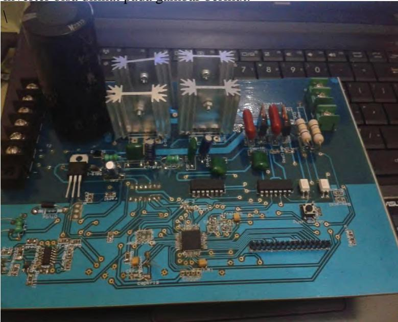
**Gambar 3.8 Modul PCB Inverter**
