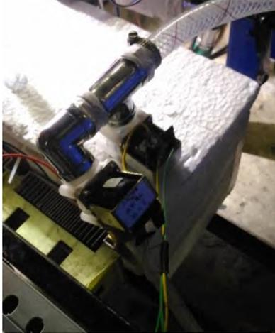
**Gambar 3.5** Solenoid 3-way Valve
